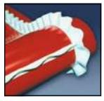
These versatile belts are fabricated with PVC and polyurethane (PU) corrugated sidewalls for a wide range of lightweight monofilament conveying applications. FDA approved and resistant to oil and animal fat, thermoplastic sidewall belts are designed for pulley diameters down to 2-3/8".
