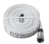
Outer construction: Single jacket, synthetic Tube construction: Thermoplastic Impregnation: Yellow Proof pressure: 300 PSI
