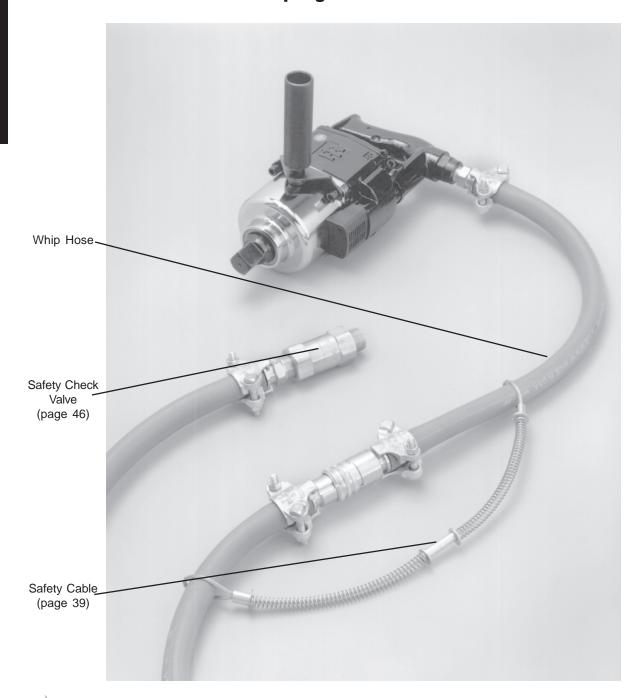
It is important to be safe when installing quick disconnect couplings into a pneumatic circuit. Never install a pneumatic coupling directly into an air tool, use a piece of hose that is at least 18" long, between the tool and the coupling, to prevent damage to the coupling. To protect the operator, safety devices, such as a Safety Check Valve (page 46) and Safety Cable (page 39) should be installed in case there is a hose or coupling failure.
