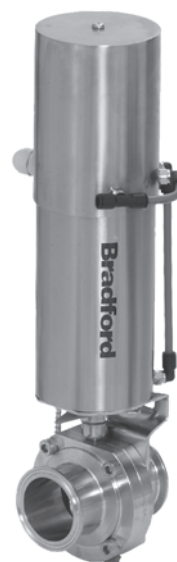
Bradford™ automated butterfly valve with vertical canister air-to-open spring-to-close actuator and control top, with 24VDC solenoid. B5101S200CC-ZB
