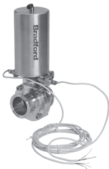
Bradford™ automated butterfly valve with vertical canister air-to-open spring-to-close actuator and proximity sensors. B5101S200CC-MI
