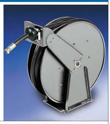
Notes: Spool hose connection fittings must be Female NPSM. Reels are primarily for manual pullout applications with lift height no more than 20ft. Otherwise, please call factory for application assistance.
