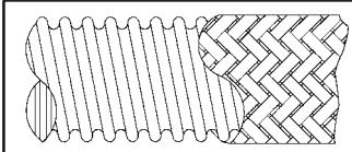
**Extraflex** is Hose Master's spirally-welded corrugated metal hose, specifically designed to maximize flexibility while maintaining good pressure ratings. The helical design facilitates draining and reduces in-line turbulence.
