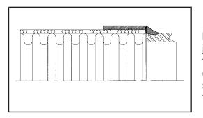
Half-Corrugation - Standard fabrication sometimes leaves a portion of the cut corrugation, or corrugation "lip", just under the base of the fitting. In specialized applications this residual lip may not be desirable. To prevent any exposed corrugation edges from causing damage, the hose can be specially prepared for welding by cutting the corrugation on the crest, rather than in the valley, thereby removing the lip.
