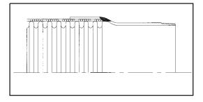
**Smooth Transition Weld** - For applications in which corrosion is a concern, all crevices and fissures must be minimized. Specialized hose and fitting preparation, in conjunction with proprietary welding techniques, is available to provide a full penetration hose-to-fitting weld that is smooth and crevice free.
