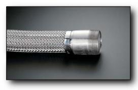
**Braid** - For higher than normal working pressures, or for critical safety situations, a stainless steel braid can be installed and welded over a stripwound hose assembly. The braid serves to prevent the hose from overextending and damaging the hose
