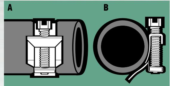
**A.** Illustrates Lox-On compression at only 20 in. lbs. tightening torque on 160 PSI (high density) polyethylene pipe. This is half the torque generally applied to conventional worm drive clamps.
