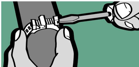
Bend band at 90° from buckle and engage outer tooth with serration. Hold band down and tighten screw.
