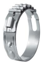
OETIKER Stepless® Low Profile Clamps 192, with tolerance compensation features accommodate dimensional variations in the parts being clamped, also when applying high radial forces. In addition, the flexible tolerance-compensation elements, consisting of up to six convolutes in the strip material are designed to allow for minor diameter changes caused by temperature variations and/or the effects of vibration.
