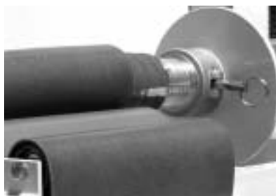
Place fitting to be inserted at the end of the hose, in front of the pneumatic ram plate.
