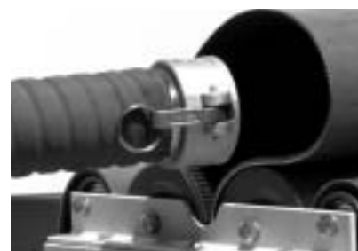
Release the tension on the gripping belt and remove the finished assembly.
