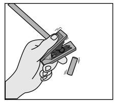
**Assembly** Cut the tube square. Debur copper tubing
