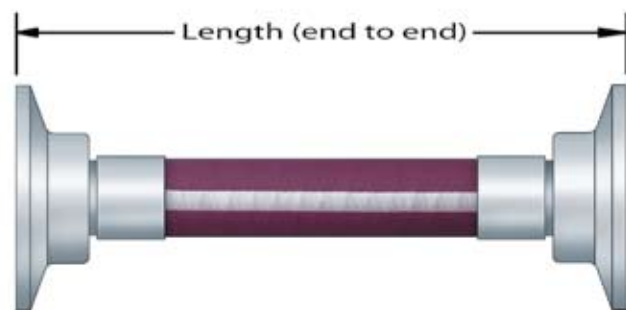
Sanitary x Sanitary Assembly
