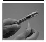
Push fitting onto hose slightly and then remove tape. Continue pushing fitting onto hose until fitting reaches depth insertion mark. (If fitting does not readily slide onto hose, perform the next step.)
