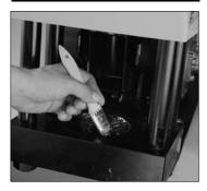
Using a molybdenum disulfide type grease, apply a thin layer of grease on bowl of crimper base plate.
