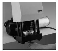
crimped or damaged fitting. Position ring so it is centered on die. Place silver die ring on top of die.
