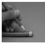
Mark hose end with proper insertion depth line. For 919U hoses, use a sharp knife and light pressure to cut back the urethane cover at least the length of the insertion depth of the fitting.
