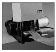
Place silver die ring on top of die. Position ring so it is centered on die. CAUTION: When positioning fitting in die, ensure fitting skirt rests on die step. Failure to do so will result in an improperly
