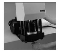
Crimp fitting onto hose until die ring contacts base plate.
