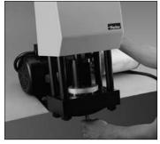
While holding hose and fitting in position on die step, pull down on handle to activate crimper.
