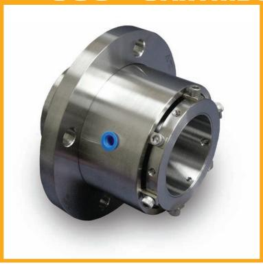
The SEPCO® CGS is a single, cartridge-mounted mechanical seal that can be used to replace double seals without using a water flush. The unique feature of the CGS Seal is a grease barrier cavity to prevent product leakage to the atmosphere without elaborate environmental controls.
