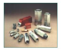
Snap-tite offers a wide range of soft seated standard inline and cartridge style check valves in plated steel or 316 stainless steel. Other materials are also available upon request as are specially designed check valves to meet specific criteria. Standard sizes range from 1/4" to2" with pressures up to 6000 psi (415 bar) and flows to 175 gpm (662 l/min).
