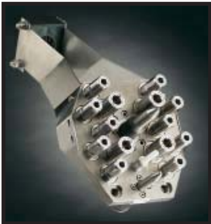
ROV installed stab plate uses PEEK sealed poppet style couplings in sizes 1/4" and 1/2" and includes guide pins to aid in alignment of the panels.
