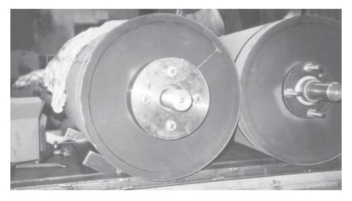
Dead shaft pulleys are different from traditional pulleys. The shaft is held fixed (dead) and not allowed to rotate. The pulley is mounted on bearings and rotates around the fixed shaft.
