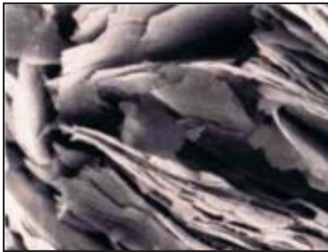
Vermiculite's thin, flexible, soft plates can be exfoliated like graphite. They retain the sealability and low porosity of graphite, but Flexitallic's new Thermiculite sheet gaskets will not oxidize at high temperatures.
