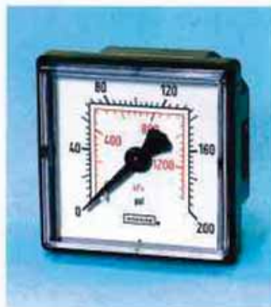
20.148 2 INCH ABS SQUARE CASE 1/8" NPT/10-32 FEMALE CENTER BACK CONNECTION PANEL MOUNT
