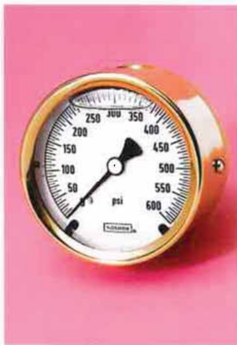
25.310 2½ INCH BRASS CASE GLYCERINE FILLED ¼" NPT CENTER BACK CONNECTION
