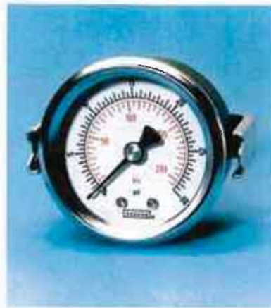
20.120 2 INCH STEEL CASE 1/4" NPT CENTER BACK CONNECTION PANEL MOUNT
