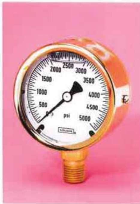
25.300 2½ INCH BRASS CASE GLYCERINE FILLED ¼" NPT BOTTOM CONNECTION
