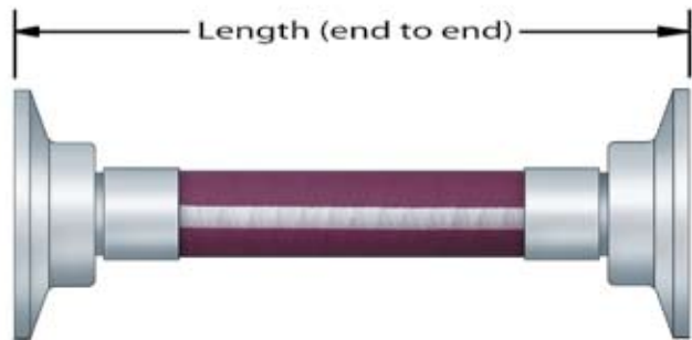
Sanitary x Sanitary Assembly
