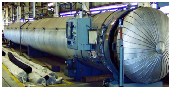
Autoclave for steam curing large diameter hoses
