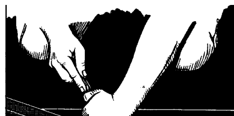
Fig. 3-3: Improper care and use of the ply lifter may also damage the adjacent ply and may
