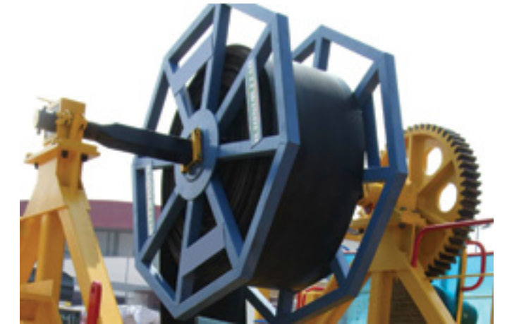
Fig. 2-5: Typical belt winder (with snub roll) set-up.
