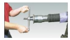
Assemble handle, ball bearing, mandrel, sleeve or pusher plate. Place hose nipple on mandrel.
