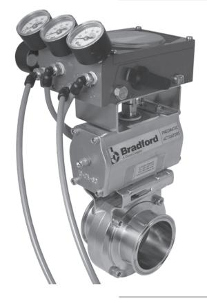
Bradford<sup>™</sup> automated butterfly valve with stainless steel horizontal rack and pinion air-to-open air-to-close actuator and pneumatic positioner, with full gauge set. **B5101S300CC-AQ**
