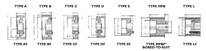
The figure following the sketch reference letter in the "Type" column indicates the construction of the sprocket (1=Solid, 2=Web, and 3=Arms), and the letter "F" indicates that the sprocket has flanges.
