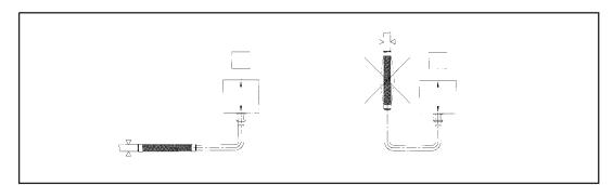
If there is vibration in more than one direction, either install a longer hose bent at 90° or install a "Dog Leg" assembly.
