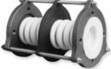
When under pressure, a longer bellows will react the same as a column when subjected to compression. At some point both will buckle or "squirm". PROCO can offer a solution to prevent this squirming effect during operation or testing.
