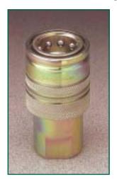
This is a dependable and economical  $1/2^{"}$  ISO 7241-1 Series A coupler which has a dual-acting sleeve. The sleeve, which has snap ring grooves that allow it to fit most industry standard brackets, permits one-hand connect or disconnect operation. This coupler is not designed for connection under pressure.
