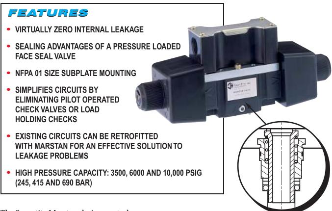
The Snap-tite Marstan design controls both static and dynamic fluids, providing many advantages through its inherent "zero leakage" feature. Marstan tight sealing internal seals assure less than four drops per minute leakage (per seal) at pressures from 0 to 10,000 psi (690 bar). The construction of Snap-tite Marstan valves is such that this "zero leakage" characteristic actually improves over time, thus increasing service life.
