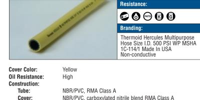
NBR/PVC, carboxylated nitrile blend RMA Class A 4-spiral polyester yarn - 1/4", 3/8", 1/2" sizes -40°F to +212°F **Temperature Range:** -40°C to +100°C Reels
