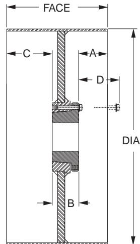
With continuously welded disc-to-rim construction and compression type hubs, VAN GORP has turned the weak link in most elevator conveyor systems into the strong point. Now, you get a super strength, one piece, single disc steel elevator pulley, superior to any other on the market today.
