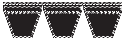
Envelope 5V, 8V Cross Section
