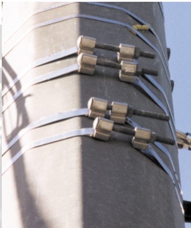
Heavy Duty Bolt Clamp used for attachments to large diameter power transmission poles. Heavy Duty Giant Band can be tensioned using common handtools. This band application can be readjusted, moved or reused.
