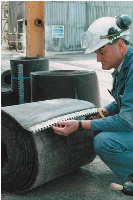
Tension is distributed evenly across the entire width of a properly squared belt, minimizing problems associated with belt mistracking and premature splice wear.
