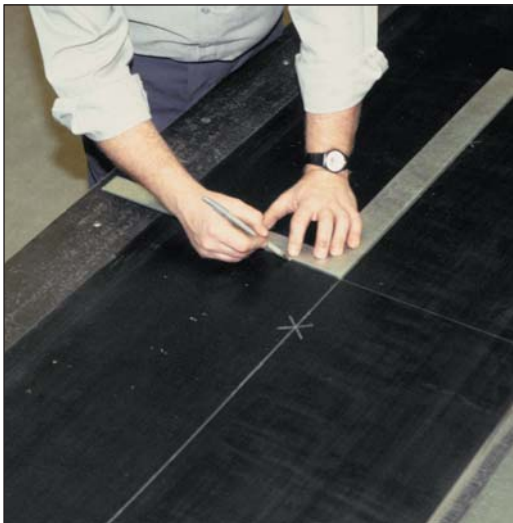
Squaring a belt end requires only common measuring tools and a Flexco belt cutter.
