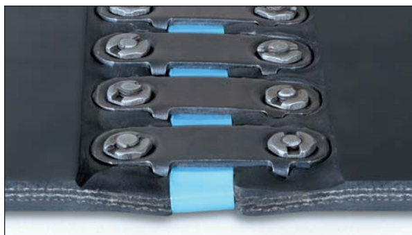
When belt top covers are 3/16" (5 mm) or more, countersinking (recessing) fastener plates is recommended.
