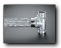
Metal hose is more versatile than other hose in that virtually any fitting can be attached to metal hose. Other types of hose require special shanks and collars in order to attach fittings. For metal hose, any fitting made from a weldable material can be attached without the need for special features. This versatility also means that multiple fittings can be welded together to make custom solutions for difficult applications.
