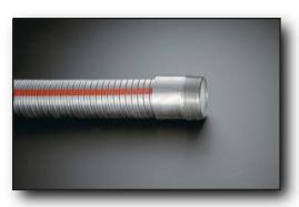
**Lay Line** - A straight, painted line can be applied to interlocked hose along its entire length. This lay line serves to give clear warning to the user if the hose is being potentially damaged from torque or twisting in service. Monitoring torsion or twisting of the assembly can significantly increase the service life of the hose.
