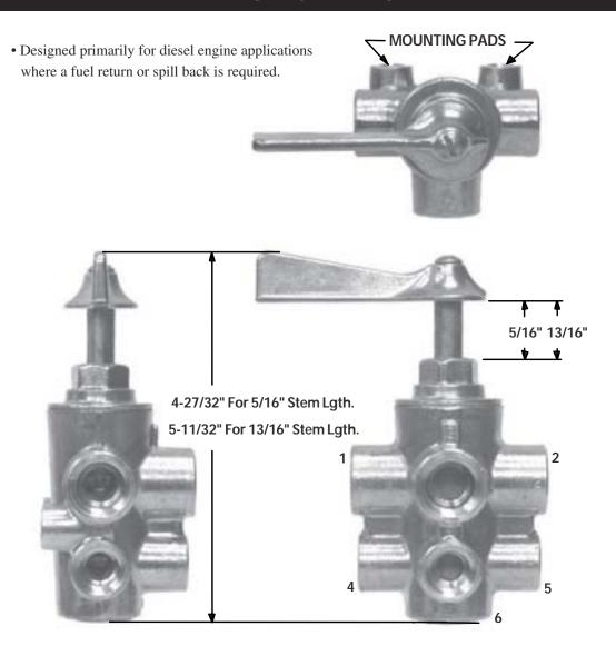
Maximum Handle Travel 180° Mounting Pads for Bolt Mounting
