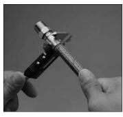
Measure crimp diameter of each fitting at top, middle and bottom of shell. Take measurements at a minimum of three places around shell circumference. Verify crimp diameter is within tolerances. (Refer to Crimp Specification & Tool Selection Chart for proper crimp diameters.)
