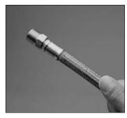
Inspect insertion depth mark at fitting ends. Insertion mark must be visible and within 1/8" of bottom of fitting shell.
