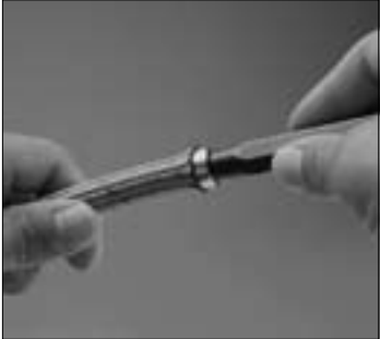
Using a tapered punch, push punch into end of sleeve and tube to set sleeve barbs into tube.
