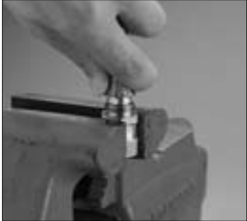
Using a twisting motion, push hose over nipple until hose is seated against nipple chamfer.
