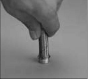
By hand, push sleeve over end of TFE core tube and under wire braid.
