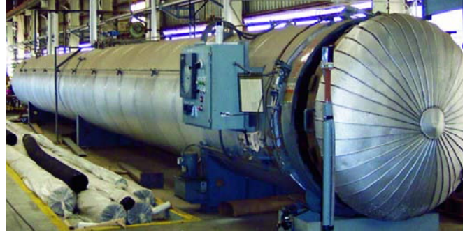
Autoclave for steam curing large diameter hoses
