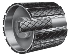
Quality rubber is bonded to special traction pads fitting the pulley rim. The pads slide into retainers welded into the pulley rim. New pads can easily be replaced without removing the pulley from the conveyor.
