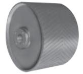
Vulcanized rubber lagging is 60±5 durometer Shore A, S.B.R. black rubber without a cloth fabric. It is bonded directly to the pulley rim in the vulcanizing process. The finished rubber surface has a cloth impression. When GROOVING is required, please specify whether herringbone or another type of grooving is desired. Normally, grooving should not be used in vulcanized rubber less than 3/8" thick.
