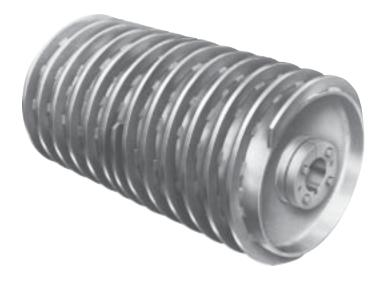
The VAN GORP® Spiral Drum Pulley is formed by a pair of vertical steel bars helically wound around a heavy-duty reinforced drum pulley (H•D•R®) and towards one another with intervals between the convolutions of each. This unique design reduces the possibility of material build-up between the belt and the pulley in applications where self-cleaning wing type pulleys cannot be used.
